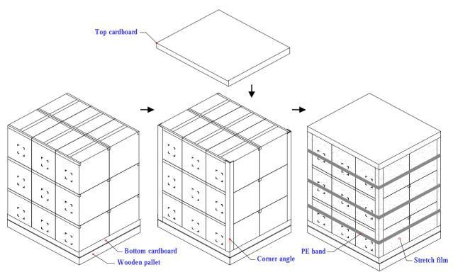
Note: Limit of box palletizing = Max 3 layers(ship and stock conditions)
